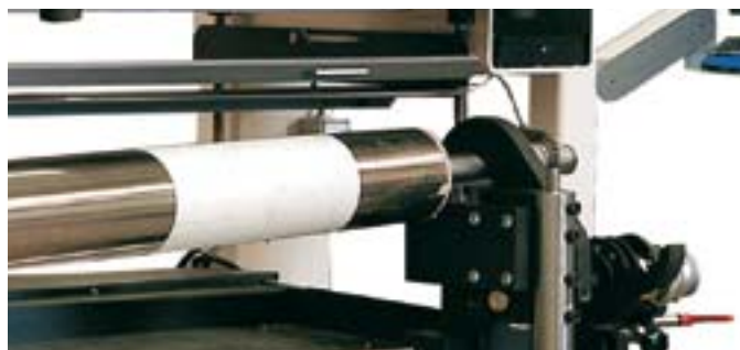
Sleeve changer on the right hand side (optional)
