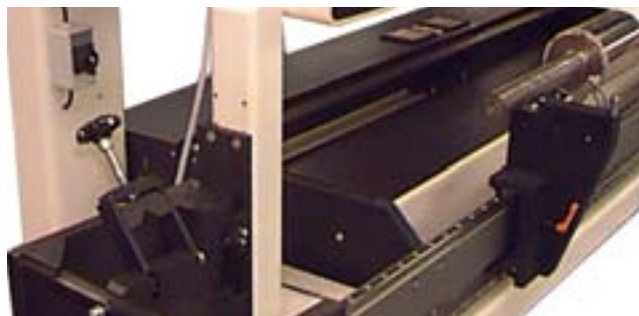
Sleeve changer on the left hand side (standard version)
