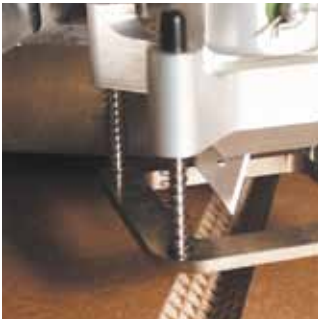
The crease wheel easily interchanges with a V-notch cutting tool, for miter cuts in triple wall corrugated.
