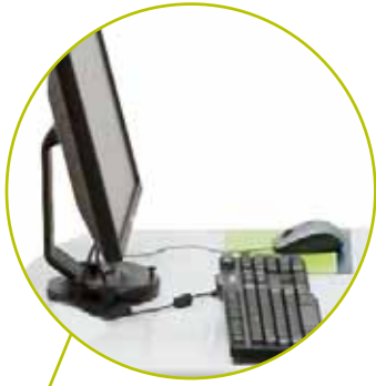
The custom operator console consists of an integrated PC workstation, screen, keyboard and operator panel.
