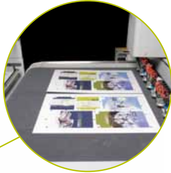
The Kongsberg i-XE10 Auto is equipped with a conveyor system for automated material processing.
