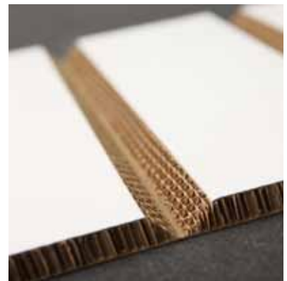
V-notch in sandwich board.
