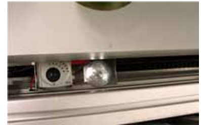
Perfect print-to-cut registration with two cameras to register marks.
